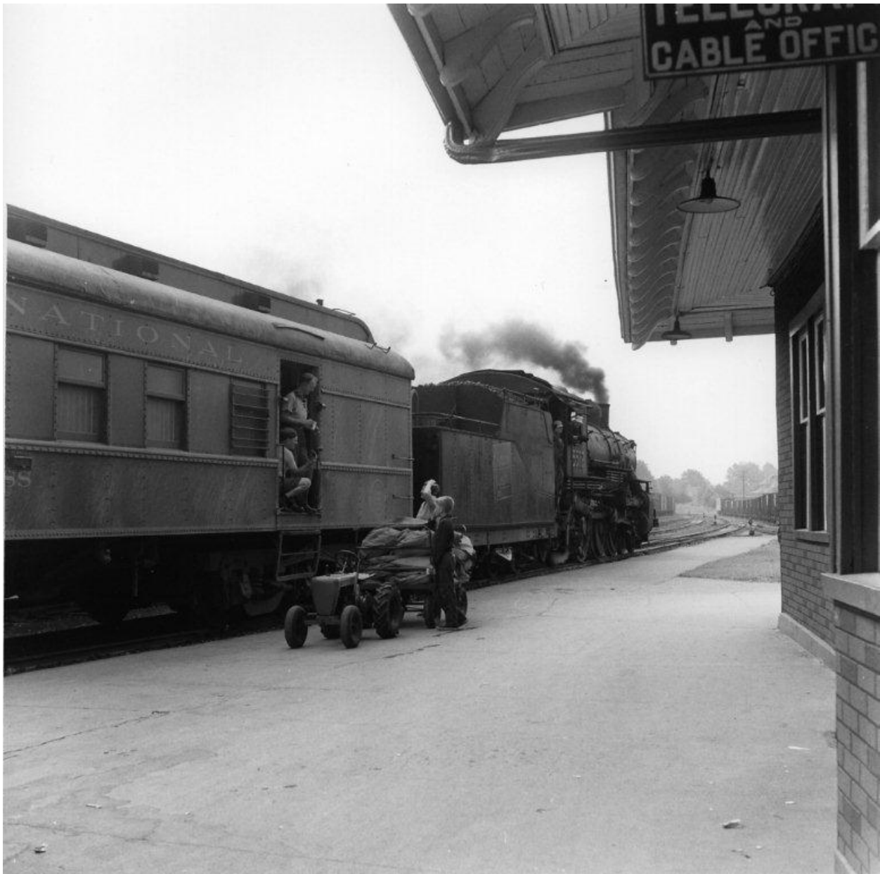
Figure 24 - Waiting, waiting for the mail at Palmerston, Ontario. This is a 30-foot Railway Post Office apartment car often used on Canadian National mail routes during the 1930s. The letter slot visible at the middle-left edge of the photograph was at the edge of the letter distribution case inside, indicating that the RPO space occupied only half of the car. Many of the RPO connections depicted in the schedules from Oshawa to Waterloo were 30-foot apartment RPOs.
