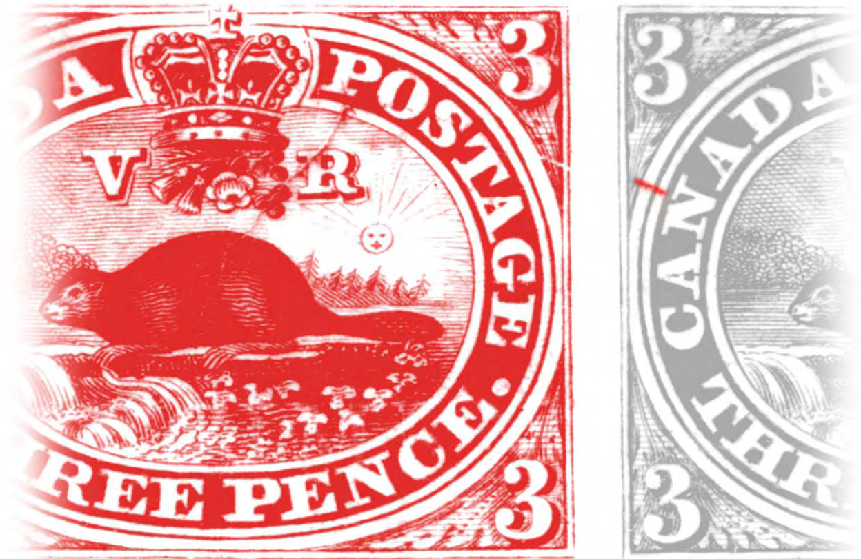
Figure 7: The first relief impression (in red) is rocked into the plate with its characteristic crack plus the small extension into the far-right margin. The second impression (in grey) is rocked in leaving the extended crack to show through as the N-flaw in the non-printing areas above the “N” of “CANADA”.
