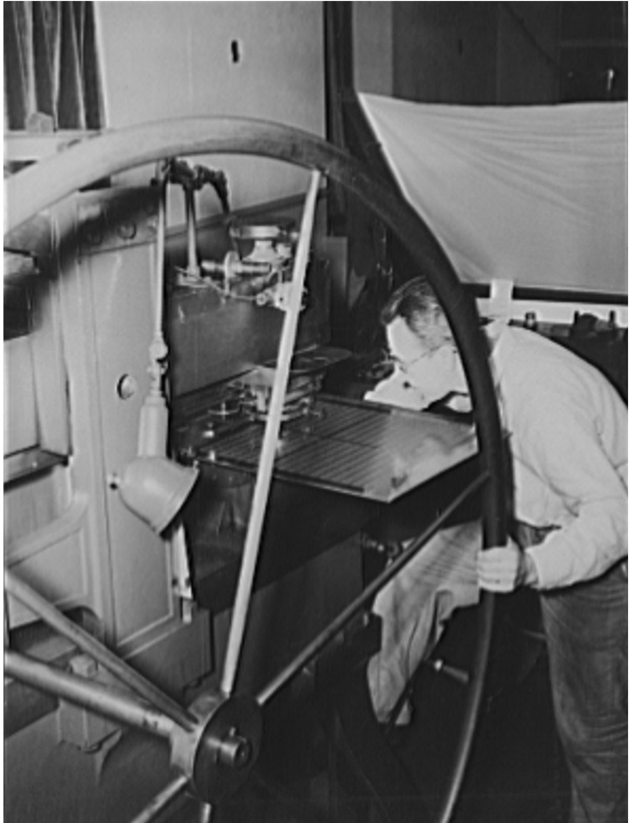
Washington, D.C. Siderographer transferring images from postage stamp transfer roll to steel plate at the United States Bureau of Engraving and Printing, Courtesy of the Library of Congress
