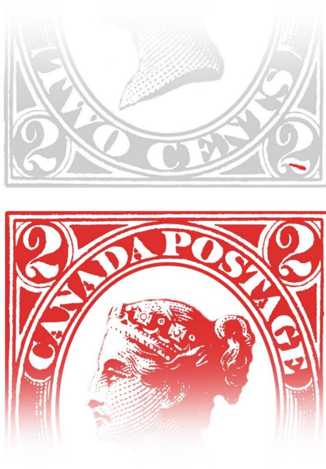
Figure 3. The first relief impression (in red) is rocked into the plate along with the dash high in the top margin. The second impression (in grey) is rocked in leaving the dash to show through in the non-printing area of the lower right 2.
