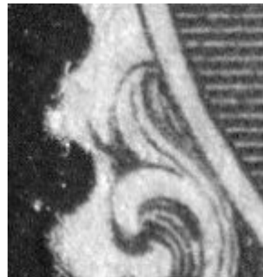
Fig. 3 More common “Spur” flaw
