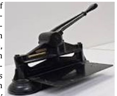
Figure 2. A Cummins Model 5 perforating machine, used to produce many of the most common perfins in Canada.
