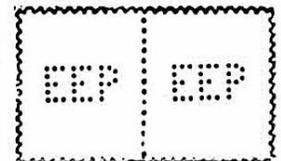
THE PERFORATIONS MADE BY THIS MACHINE CONFORM TO THE REQUIREMENTS OF THE POST OFFICE DEPARTMENT; i.e., HOLES NOT OVER 1/16 INCH IN DIAMETER, TOTAL SPACE NOT OVER 1/2 INCH SQUARE.
