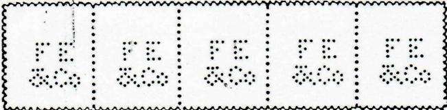
THE PERFORATIONS MADE BY THIS MACHINE CONFORM TO THE REQUIREMENTS OF THE POST OFFICE DEPARTMENT; i. e., HOLES NOT OVER  $\frac{1}{32}$  INCH IN DIAMETER, TOTAL SPACE NOT OVER  $\frac{1}{2}$  INCH SQUARE.
