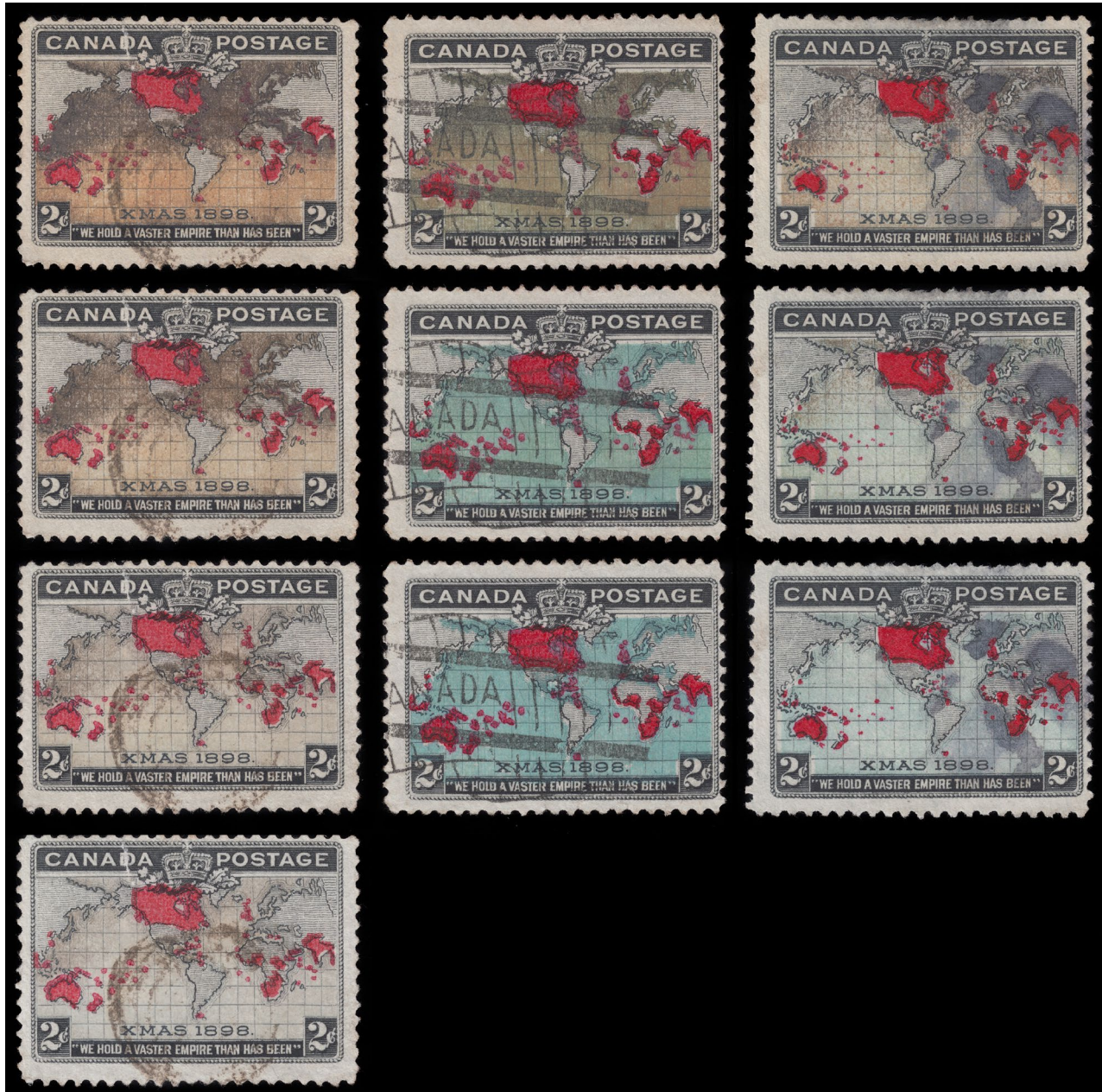
Figure 4: Illustrating the progression of three stamps treated with hydrogen peroxide. The first row is the original stamps with strong muddy waters. The second row shows the same stamps after 6 hours of fumigation. The third row shows the stamps after 12 hours of fumigation. The single stamp in the fourth row shows the stamp after it has also been soaked overnight in hydrogen peroxide solution.
