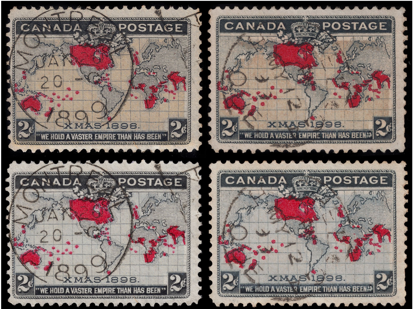
Figure 3: Example showing two used Map stamps at top before treatment and the same stamps at bottom after six hours of fumigation with 3% hydrogen peroxide solution.
