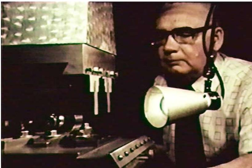
Figure 4. Siderographer Murdo Stewart transfers the image from the die to a transfer roll. [Source: *More Than Just a Pretty Face*]
