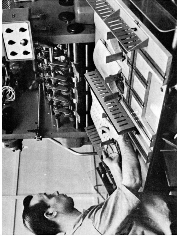
Figure 14. The panes are delivered in lots of five to the receiving trays where the top pane is press-examined. After 20 deliveries, the tray table positions the empty trays to receive the next 100 panes. [Source: *The Postmark*]
