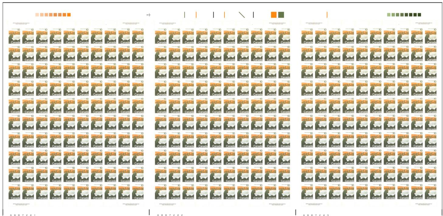
Figure 33. Digital reconstruction of the plate proof of the 1972 10¢ Landscape definitive. The low value definitives had two panes side by side on the web, but the 1972 Landscape medium value definitives had just a single pane. Note the marginal markings in the selvage that was cut away by the slitters. A security control number appears in the bottom selvage below the left side of each pane. [Source: Robin Harris]
