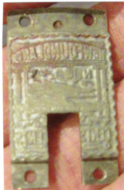
Heavy worn die removed from meter #13 George Neal Ltd. machine empty area at bottom is where value figure would be entered
