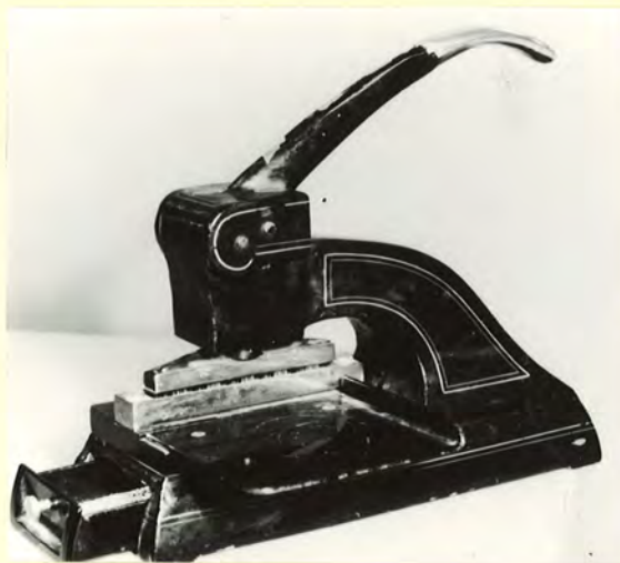
Cummins Perforator Company Model 52 was used by the Department of Finance for 5-hole OH/MS stamps.
