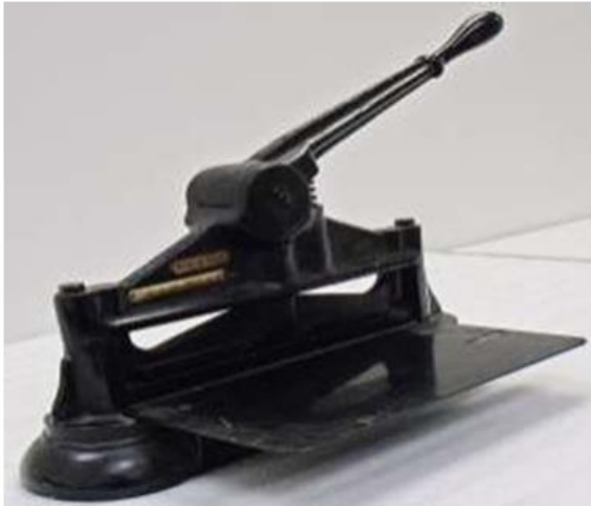
Figure 7. A Cummins Model 53 perforating machine, used to produce many of the most common perfins in Canada.
