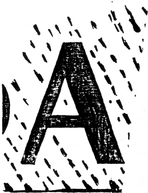
FIGURE 12. Poor inking at the right frame. Not associated with the wear of inking rollers shown in the other figures
