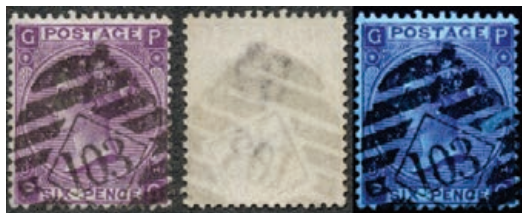
Figure 4. Great Britain stamp (1869, SG 109) printed with the first commercially available aniline dye – mauve (left). There is no bleed through (centre) and no fluorescence under UV (right).
