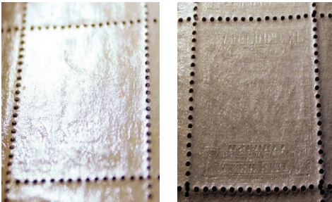
Figure 5. Embossing on the gum surface is (left) absent from stamps printed by the wet process used by Perkins Bacon, but (right) present in stamps printed by the dry process by Waterlow.
