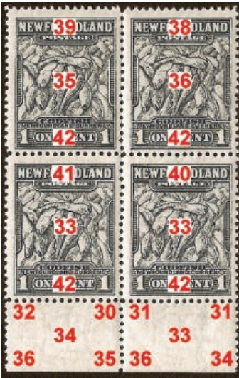
Figure 2. 1942-1948 1¢ (Scott 253) after gum removal showing variation in thickness ( \times 0.0001 ”).
