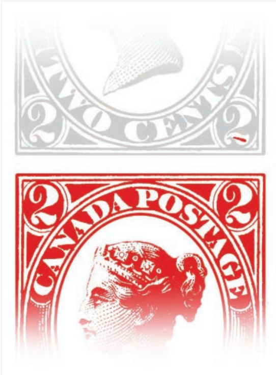
Figure 4. The first relief impression (in red) is rocked into the plate along with the dash high in the top margin. The second impression (in grey) is rocked in leaving the dash to show through in the non-printing area of the figure, lower right 2.
