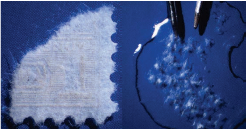
Figure 2. 1932 1c Green (Scott 183) after sixty minutes in one percent sodium hydroxide and (b) paper disintegrated with the help of needles.
