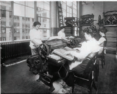
Figure 1. Rotary wheel perforator (7.95). (US Library of Congress Digital Library)
