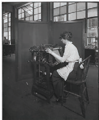
Figure 2. Rotary Bar Perforator (7.85). (US Library of Congress Digital Library)
