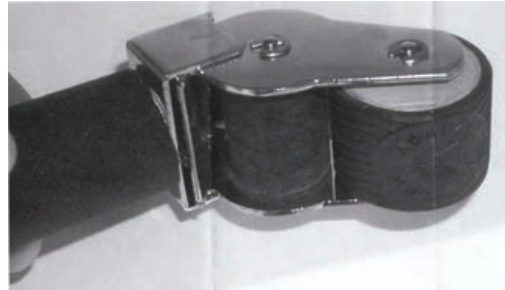
Figure 3. Close-up of the head of a “Wing” hand roller canceller. (Courtesy Canada Post).
