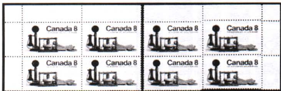
Figure 7. Misalignment of T-comb perforator
